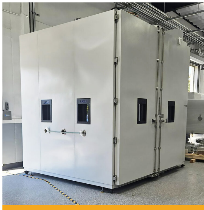
This thermal chamber is used to test EV chargers under a range of environmental conditions, helping ensure reliability and performance across all operational scenarios.
