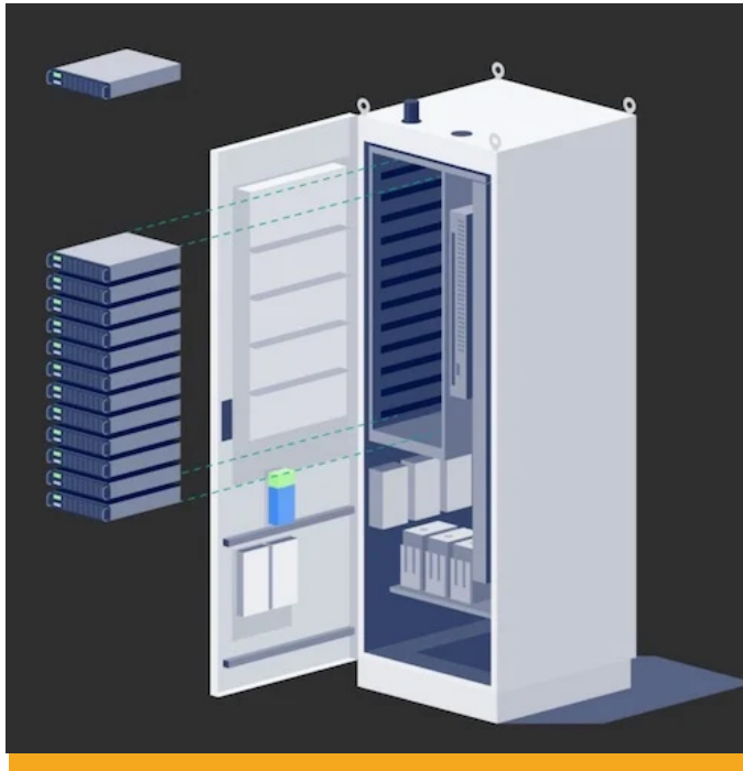
Figure 2. Technicians can increase the charging capacity of an EV charger in the field by adding additional power modules.
